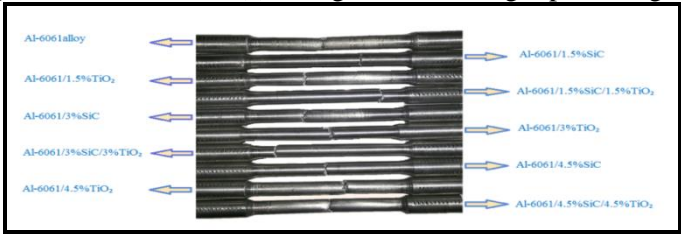
Fig(19) The samples after tensile test.
