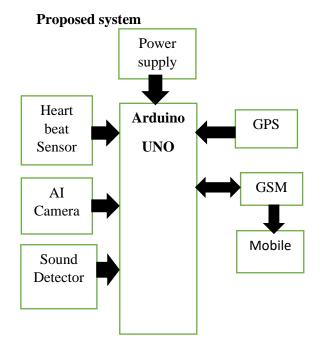
The figure above reflects the device proposed. The device consists of the Heartbeat Sensor, which monitors the speed of the heartbeat. It automatically switches on the AI camera to check the environment when the heartbeat rate reaches the specified threshold level and also recognises the victim's facial expression at that time. The Sound Detector is also activated when
