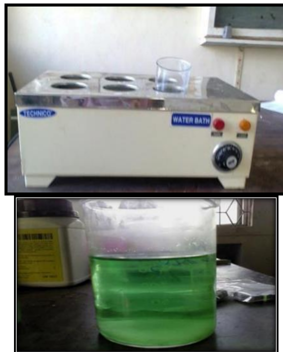
Figure3. Experimental set up used for EN deposition. Figure4. Bath preparation for the test.
