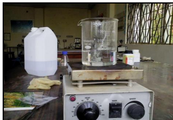
Figure2. Alkaline cleaning setup.
