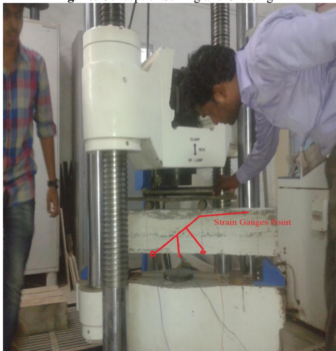
Fig. 11. Beam section Testing Set Up
