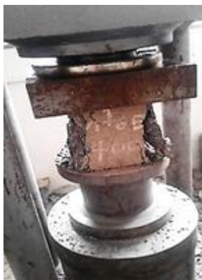
Figure 3: M 65 grade cube subjected to elevated temperature 400°C
