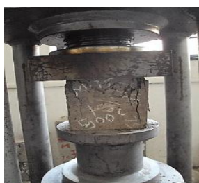
Figure 4: M 65 grade cube subjected to elevated temperature 400°C
