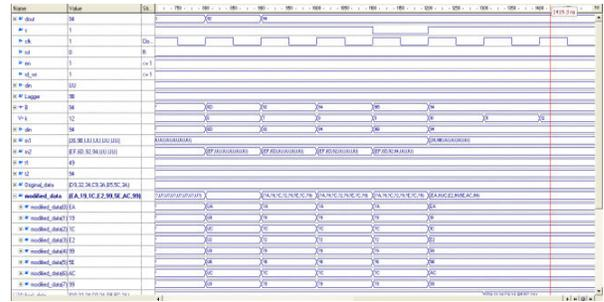
**Fig. 4: Delay instruction allocation at arbiter unit**
