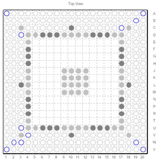
**Fig. 10: Pin layout of the implemented design for the targeted FPGA**
