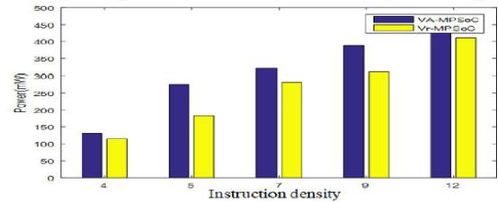
**Fig. 11: Comparison of power utilization for different instruction density**
