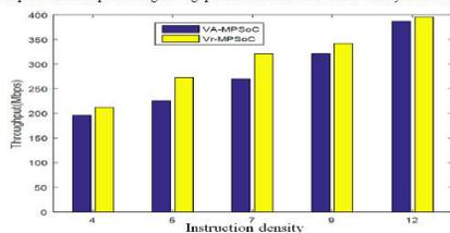
Fig. 13: Comparison of the processing throughput for different instruction density
