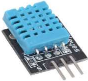
Fig .4 Temperature/Humidity Sensor (DHT11)
