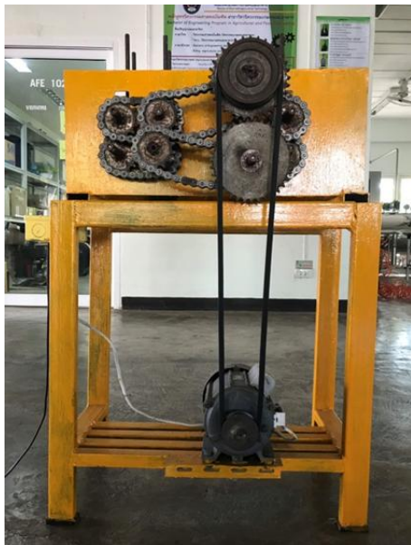
Fig. 2 Power unit and power transmission of the bamboo stripping machine
