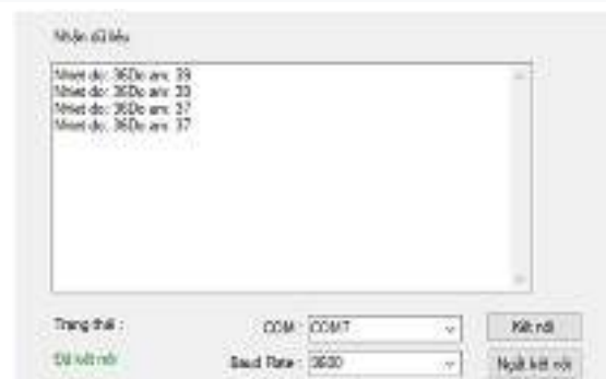
Hình 5. Windows forms interface to create applications to receive data via COM port
