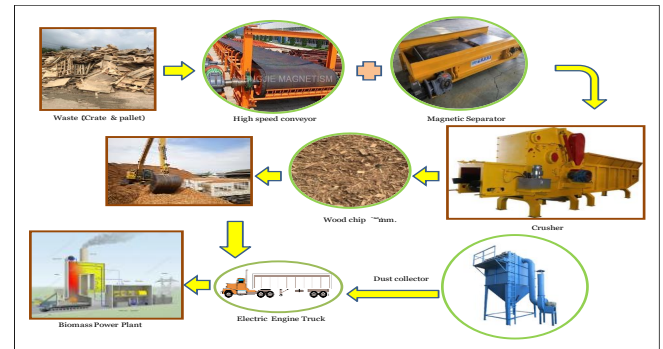
Figure 4 New findings in the wood crate waste management process into renewable energy to generate electricity
