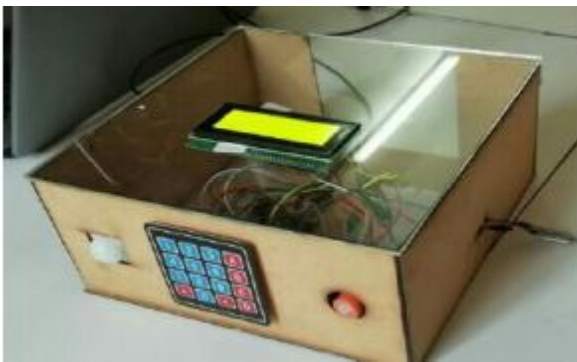
Fig.8. Project kit –Food ordering and quality checking system
