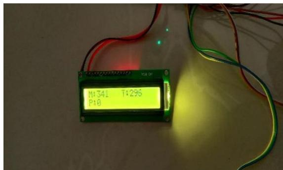
Fig.6 Display of temperature and pressure values
