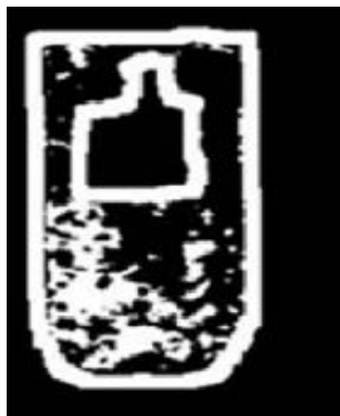
Fig 5: Hole filling and reference line matching The following figures shows the images with cap present.
