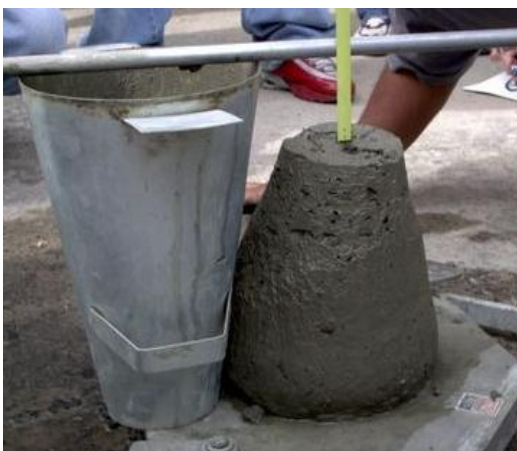
Fig. 2 Slump Test frustum Specification
